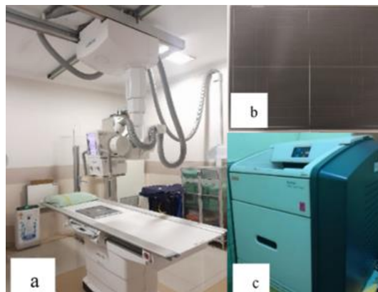
Gambar 1. Pesawat sinar-X Digital Radiography (DR) merk Siemens (a), detector ukuran 35 x 45 cm (b), printer (c). (RSUD Kota Yogyakarta, 2025)
